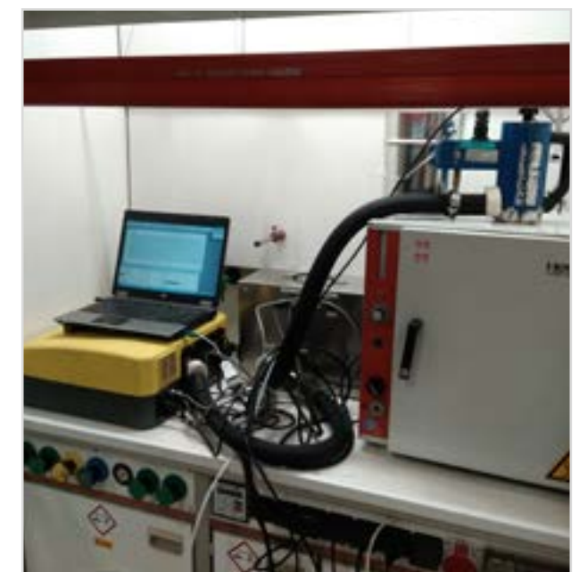
Foto 5: FTIR (Fourier Transform Infrared) Gasanalysator
